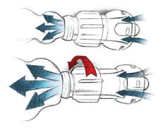
The swivel nozzle is fully adjustable with the intensity of the flow can be fully regulated – in either direction.
